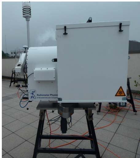
RPG-HATPRO-G5 radiometer during the absolute calibration procedure.
